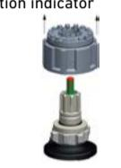
9. Push spindle device out of the inner housing with a little tap on the position indicator
