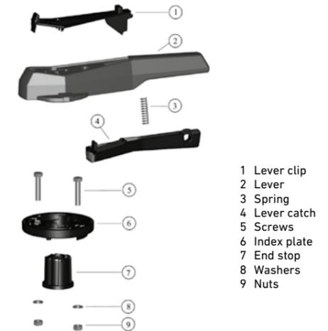
1. Hand lever should be assembled with disc closed. By the indication of the shaft and the end stop a clear assembly is ensured.
