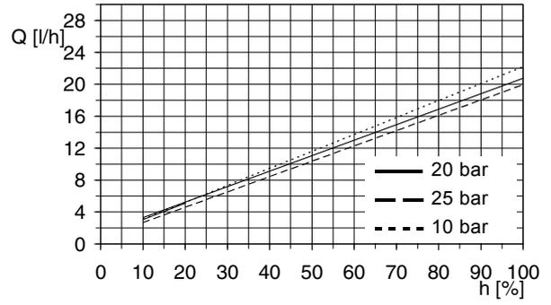
Fig. 63 DMH 17-25 (50 Hz),  $Q_0 = 20$  bar
