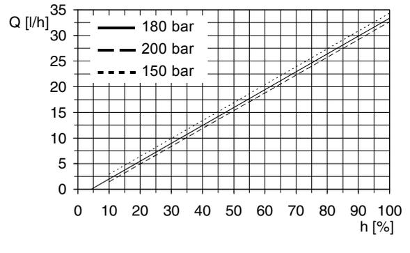
Fig. 58 DMH 23-16 (60 Hz),  $Q_0 = 10$  bar
