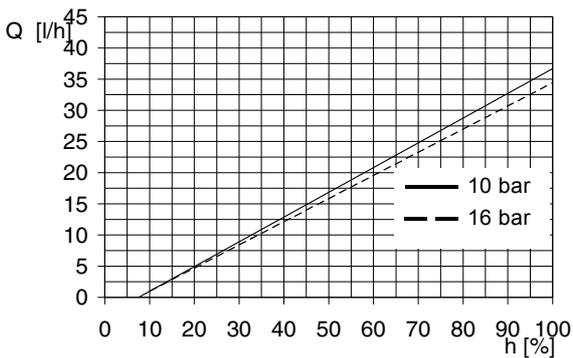
Fig. 77 DMH 36-16 (50 Hz),  $Q_0 = 10$  bar
