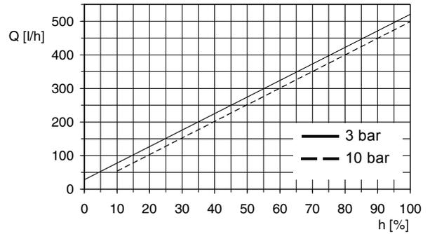
Fig. 116 DMH 403-10 (60 Hz), Q<sub>0</sub> = 3 bar
