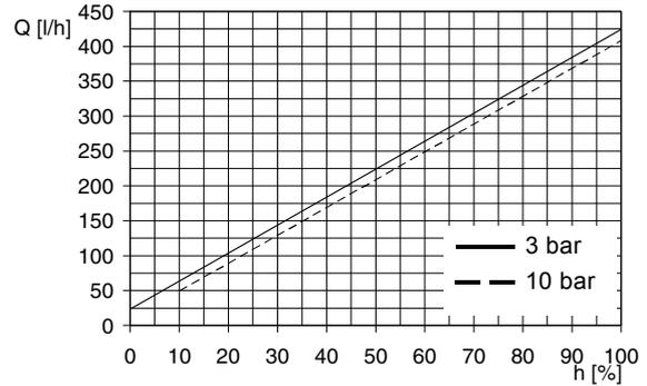
Fig. 114 DMH 332-10 (60 Hz), Q<sub>0</sub> = 3 bar
