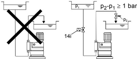
**Fig. 18** Installation to avoid the siphon effect
