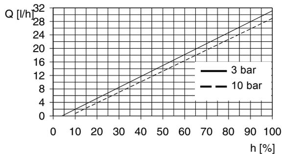
Fig. 69 DMH 24-10 (60 Hz),  $Q_0 = 3$  bar
