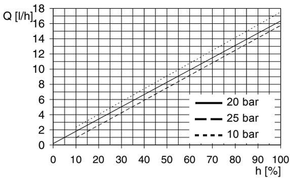
Fig. 62 DMH 11-25 (60 Hz),  $Q_0 = 20$  bar
