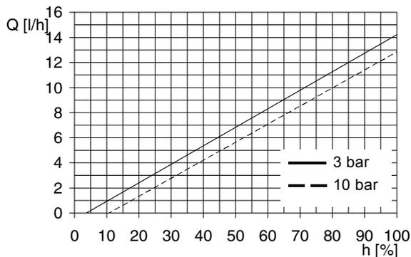
Fig. 67 DMH 11-10 (60 Hz),  $Q_0 = 3$  bar
