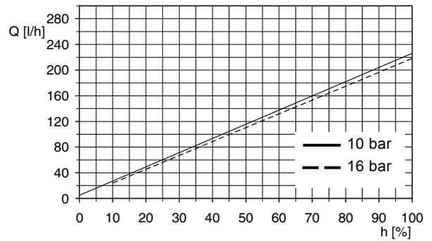
Fig. 106 DMH 202-16 (50 Hz),  $Q_0 = 10$  bar
