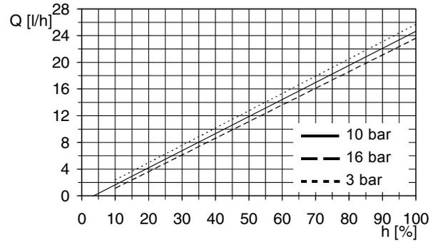
Fig. 56 DMH 18-16 (60 Hz),  $Q_0 = 10$  bar
