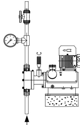
**Fig. 28** Setting the opening pressure
