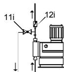
Fig. 11 Installation with ball valve and non-return valve
