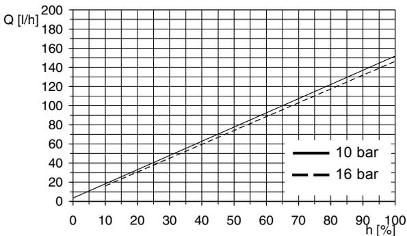
Fig. 102 DMH 136-16 (50 Hz),  $Q_0 = 10$  bar
