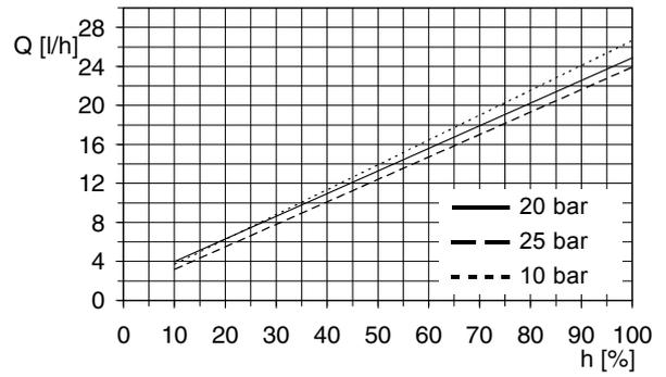
Fig. 64 DMH 17-25 (60 Hz),  $Q_0 = 20$  bar
