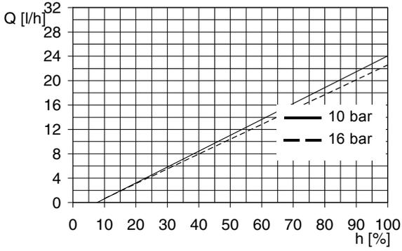
Fig. 75 DMH 23-16 (50 Hz),  $Q_0 = 10$  bar
