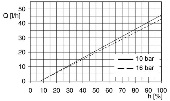
Fig. 79 DMH 45-16 (50 Hz),  $Q_0 = 10$  bar
