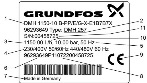
Fig. 1 DMH nameplate
