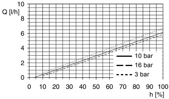
Fig. 51 DMH 4.9-16 (50 Hz),  $Q_0 = 10$  bar
