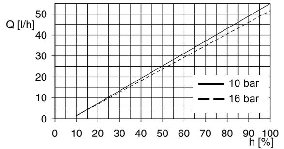
Fig. 80 DMH 45-16 (60 Hz),  $Q_0 = 10$  bar
