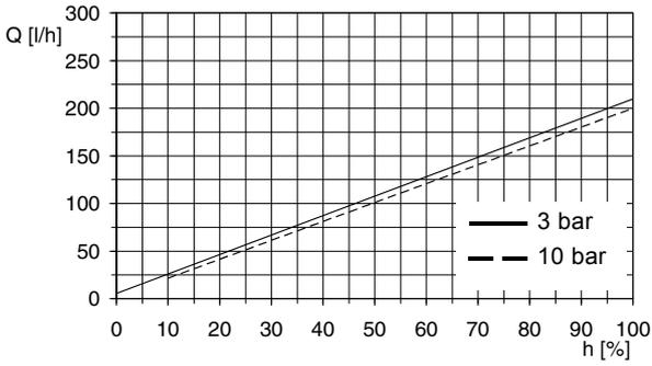
Fig. 109 DMH 194-10 (50 Hz), Q<sub>0</sub> = 3 bar
