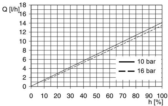
Fig. 53 DMH 12-16 (50 Hz),  $Q_0 = 10$  bar
