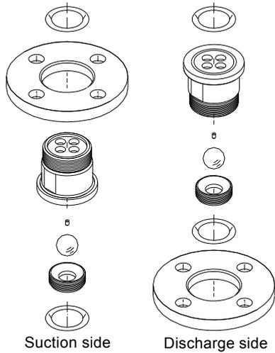
Fig. 36 DN 32 valve, suction side and discharge side
