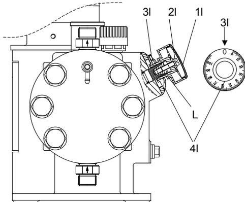
Fig. 31 Setting the dosing capacity
