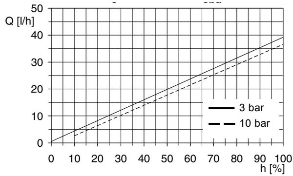
Fig. 70 DMH 37-10 (50 Hz),  $Q_0 = 3$  bar
