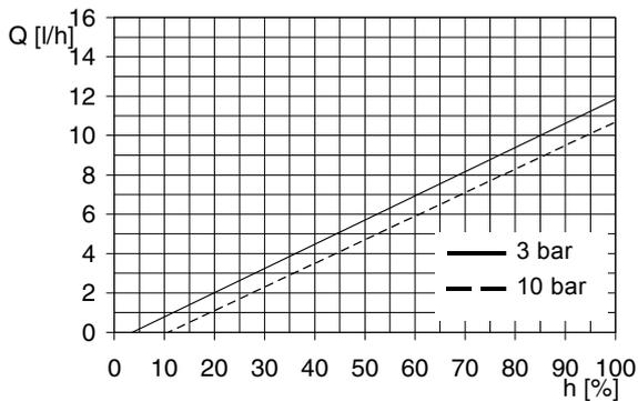
Fig. 66 DMH 11-10 (50 Hz),  $Q_0 = 3$  bar
