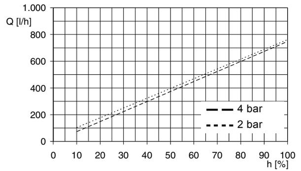
Fig. 124 DMH 750-4 (50 Hz),  $Q_0 = 3$  bar
