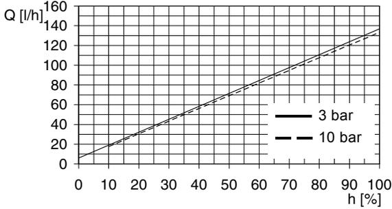
Fig. 92 DMH 102-10 (60 Hz),  $Q_0 = 3$  bar
