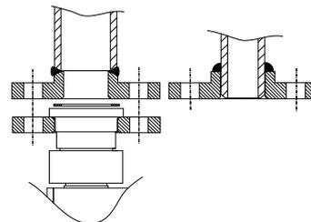
**Fig. 21** Connection of DN 32 pipe lines
