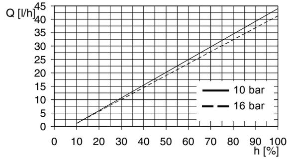
Fig. 78 DMH 36-16 (60 Hz),  $Q_0 = 10$  bar
