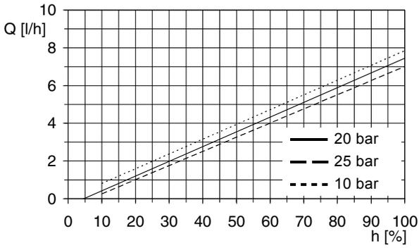
Fig. 60 DMH 4.5-25 (60 Hz),  $Q_0 = 20$  bar
