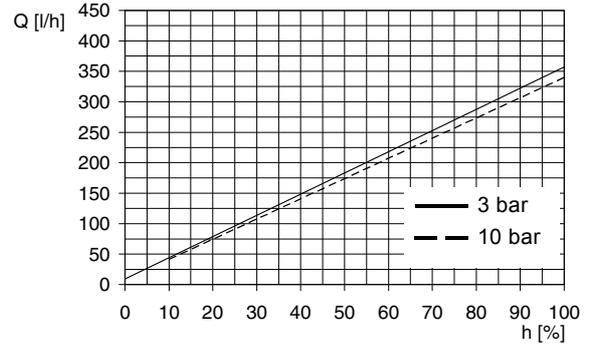
Fig. 113 DMH 332-10 (50 Hz), Q<sub>0</sub> = 3 bar
