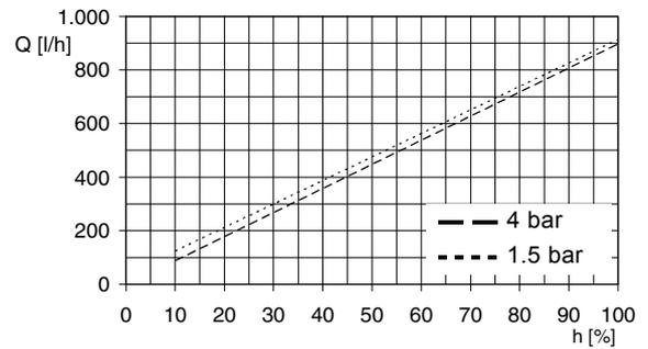
Fig. 125 DMH 750-4 (60 Hz),  $Q_0 = 3$  bar
