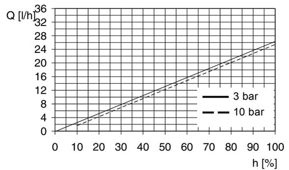
Fig. 50 DMH 24-10 (50 Hz),  $Q_0 = 3$  bar
