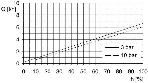
Fig. 44 DMH 5-10 (50 Hz),  $Q_0 = 3$  bar
