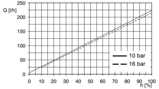
Fig. 105 DMH 166-16 (60 Hz),  $Q_0 = 10$  bar
