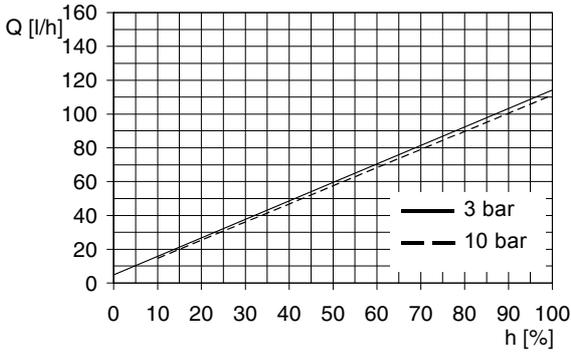
Fig. 91 DMH 102-10 (50 Hz),  $Q_0 = 3$  bar
