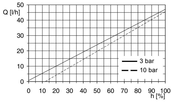
Fig. 71 DMH 37-10 (60 Hz),  $Q_0 = 3$  bar
