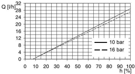
Fig. 76 DMH 23-16 (60 Hz),  $Q_0 = 10$  bar
