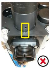
Now the autobrush for automatic cleaning can be mounted. Make sure that it is aligned with the notches correctly. After insertion fasten the grey union nut.
