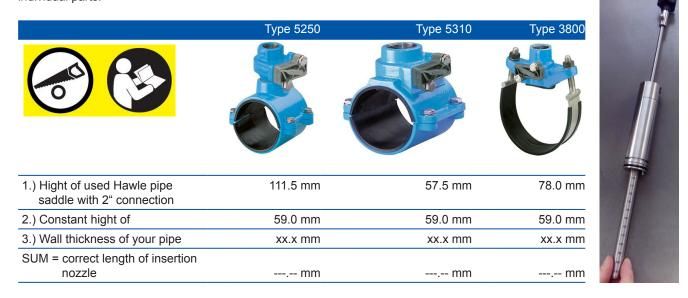
Example: If Type 3800 is used and wall thickness of pipe is 10.0 mm, then the correct lengh is 147.0 mm.
